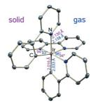
The gas-phase structure of the classical OLED triplet emitter compound fac-Ir(ppy)<sub>3</sub> was determined and a hitherto unknown, second modification of the compound was obtained by sublimation. Possible implications for an accurate quantum-chemical description of the electronic structure and some results from prior investigations are discussed in the light of the new results
